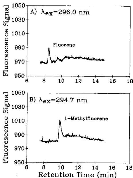
Fig. 5. Fluorescence excitation chromatograms resulting from 2- $\mu$ l injections of a hydrothermal oil sample taken from the Guaymas Basin seabed in the Gulf of California.
