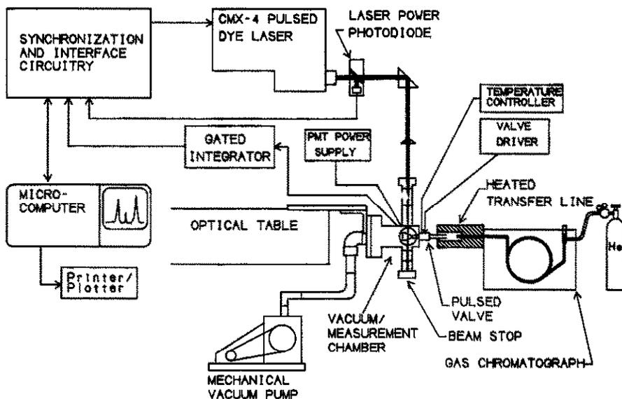
Fig. 1. Block diagram of the gas chromatography-laser-excited fluorescence-supersonic jet expansion experimental system.
