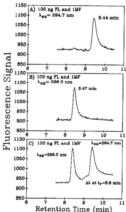
Fig. 4. Fluorescence excitation chromatograms of a mixture of 100 ng each of fluorene (FL) and 1-methylfluorene (IMF) acquired at fixed wavelengths of (A) 294.7 nm and (B) 296.0 nm, and (C) the chromatogram of the same mixture produced by a programmed excitation wavelength scan.
