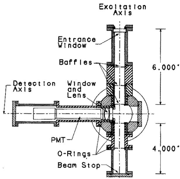
Fig. 2. Front view (looking down the expansion axis) of the supersonic jet expansion measurement cell. The supersonic nozzle and front flange are not shown.
